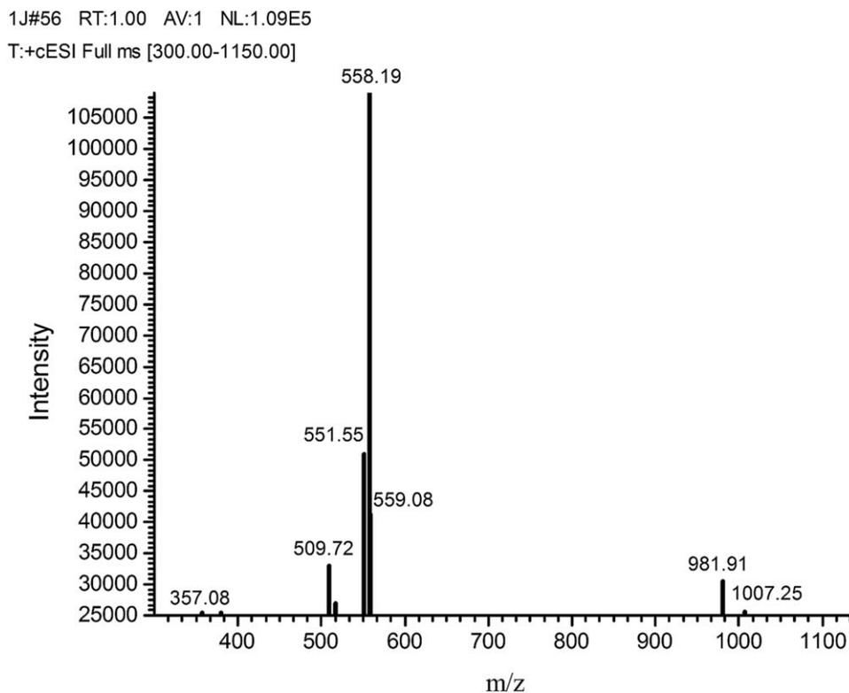
**Fig. 3.** Mass spectrum of H<sub>2</sub>N-MC-RR. The double precursor ion is at *m/z* 558.2, which is consistent with the theoretical calculated value.
